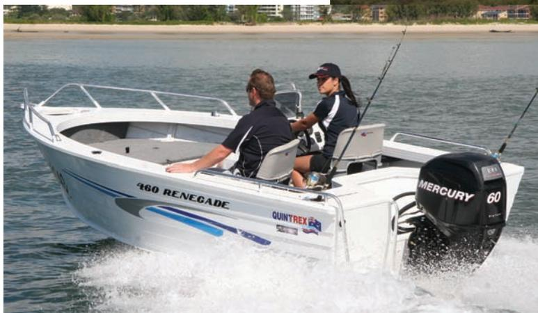
The top speed was slightly higher at full revs (5600rpm) but basically you could say the boat does a top speed around the 25-26 knots' level, which is fast enough for most fishing needs.
